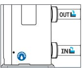
Screw back the drain plug and pipes or block them with rags so as to prevent any foreign bodies from getting into the circuit.
